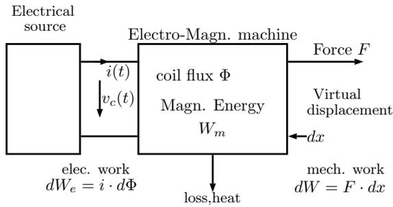
**Fig. 9:** A generalised single coil electromagnetic machine considered for a virtual displacement  $dx$  at constant current  $i(t)$ . The machine acts with a force  $F$  resulting in a work  $dW = F \cdot dx$  and consumes electrical energy  $dW_e$  whilst storing magnetic energy  $dW_m$ .
