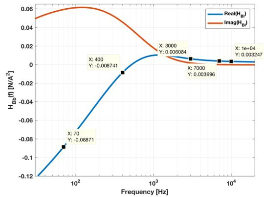
**Fig. 4:** Real and Imaginary components of  $H_{BI}(f)$  for  $x = 0$  from MagNet simulations of the 4" test driver.
