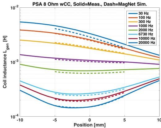
**Fig. 2:**  $|L_{gen}(f, x)|$  plotted versus  $x$  with  $f$  as parameter. Solid: measurements, Dashed: MagNet simulations.
