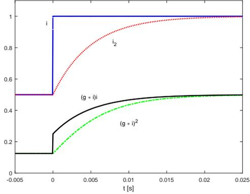
**Fig. 8:** Currents in the  $L_2R_2$  model and force contributions for  $L_2$  calculated directly on  $L_2$  ( $(g * i)^2$ ) and via the network impedance ( $(g * i)i$ ).
