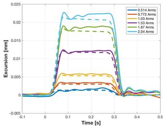
**Fig. 5:** DC-excursion caused by a series of 7 kHz tone bursts of varying amplitude with a 4<sup>th</sup> order 20Hz low-pass filter applied. Solid=measured, Dash=model fit.
