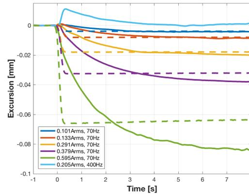
**Fig. 6:** DC-excursion caused by a series of 70 Hz tone bursts of varying amplitude and a single 400 Hz burst. All plots filtered by a 4<sup>th</sup> order 20Hz low-pass filter. Solid=measured, Dash=model fit.
