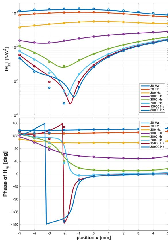
**Fig. 3:** The force factor modulation transfer function  $H_{BI}(f, x)$ , Solid: from the simulated  $Z_b$ , Round markers: from the simulated force.
