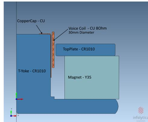
**Fig. 1:** Cross section of motor structure of the used 4" driver. The motor has rotation symmetry around the  $x$ -axis indicated by a vertical line.
