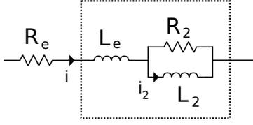
**Fig. 7:** Model of blocked voice coil impedance using the  $L_2R_2$  model. Dashed box indicate inductive part of impedance.
